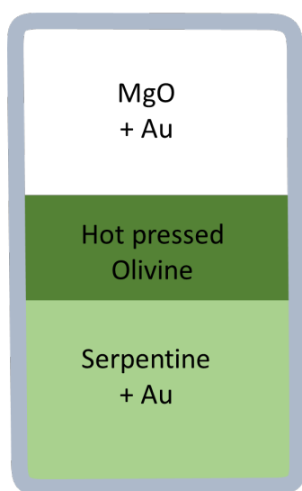
Fig. 3.8-3: Schematic of the 2 mm diameter cylindrical titanium metal capsule. The serpentinite fluid source was mixed with 5 wt. % Au powder. As the serpentine breaks down fluid is released which passes through the hot-pressed olivine core. H 2 O passing through the olivine sample transforms the MgO material above the sample to brucite. The MgO layer also contains powdered Au as a pressure calibrant. The overpressure is determined as the difference in pressure recorded by the Au in the serpentine and MgO layers.
